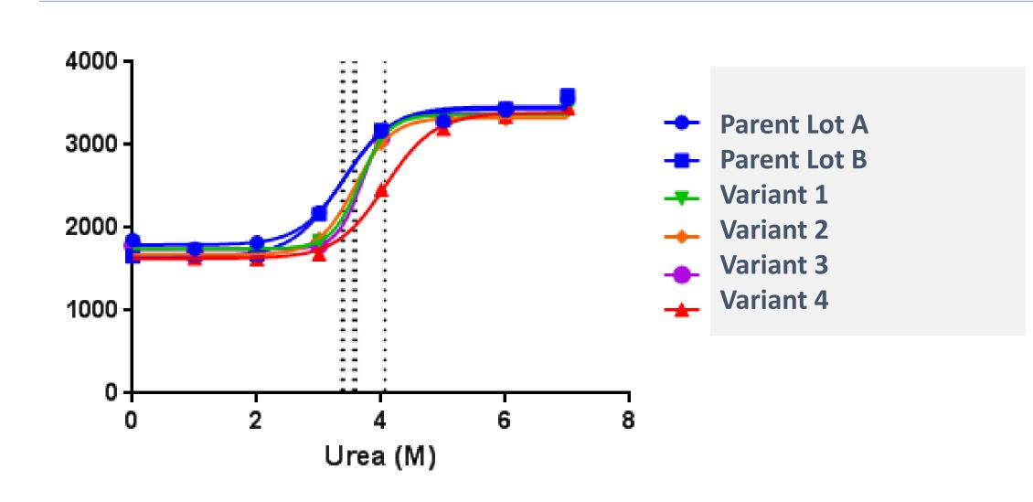
The parent ADAPTIR and optimized variants were evaluated for their resistance to denaturation by increasing concentrations of urea. In addition to increased Tm (data not shown), the variants showed greater resistance to unfolding by urea, based on the shift in EC50 values derived from urea titrations up to 7 M.
