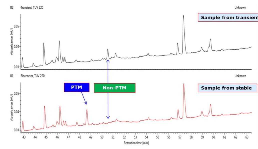
In the final stage of screening, constructs are tested by LC-MS and peptide mapping to confirm that the expected MW is achieved. In this example, proline hydroxylation occurred during stable, but not transient expression. This was addressed through sequence modification to replace the problematic residue.
